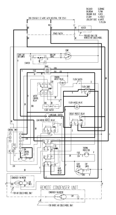
[i] When 208-230V are supplied to Circuit Protect Relay, it protects the circuit from miswiring. If the power supply is properly connected, the contact of Circuit Protect Relay does not move even when the coil is energized.
