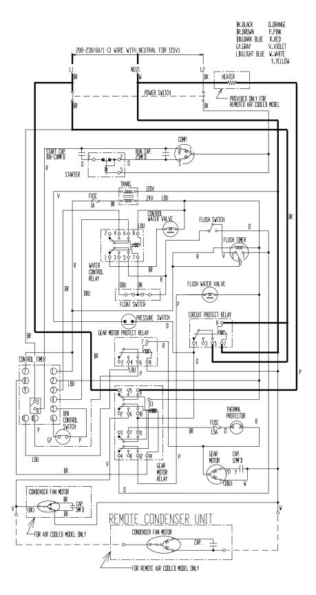
[g] When Flush Switch is moved to "FLUSH" position, Flush Water Valve opens and flushes Reservoir and Evaporator.
