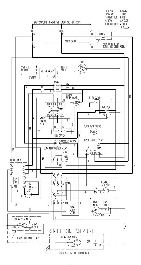
[f] Low Water (Water-cooled Model), or Dirty Air Filter (Air-cooled Model), Pressure Switch to "OPEN", Compressor and Gear Motor operates intermittently.
