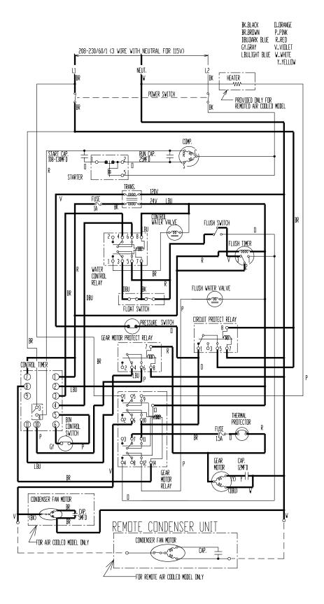
[c] Compressor starts about 60 sec. after Gear Motor starts.
